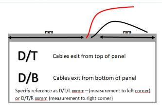
Note- measurements are always on the lit side of a panel.
